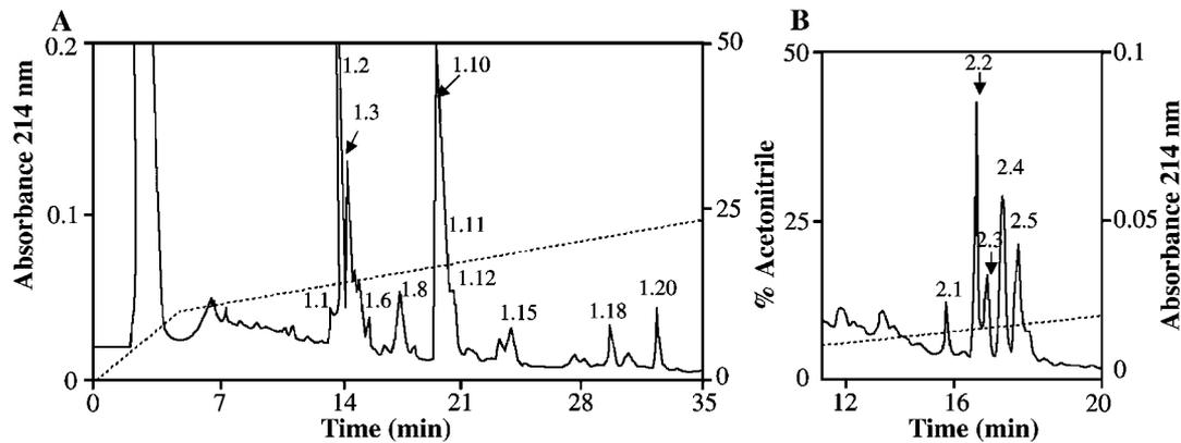
**Figure 3** Reversed-phase HPLC purification of the pooled fractions of *Agalychnis calcarifer* from zones A and B in Figure 2. Fractions were applied to an analytical Vydac C18 column as described in materials and methods. Absorbance was monitored at 214 nm. The dashed lines show the concentration of acetonitrile in the eluting solvent.
